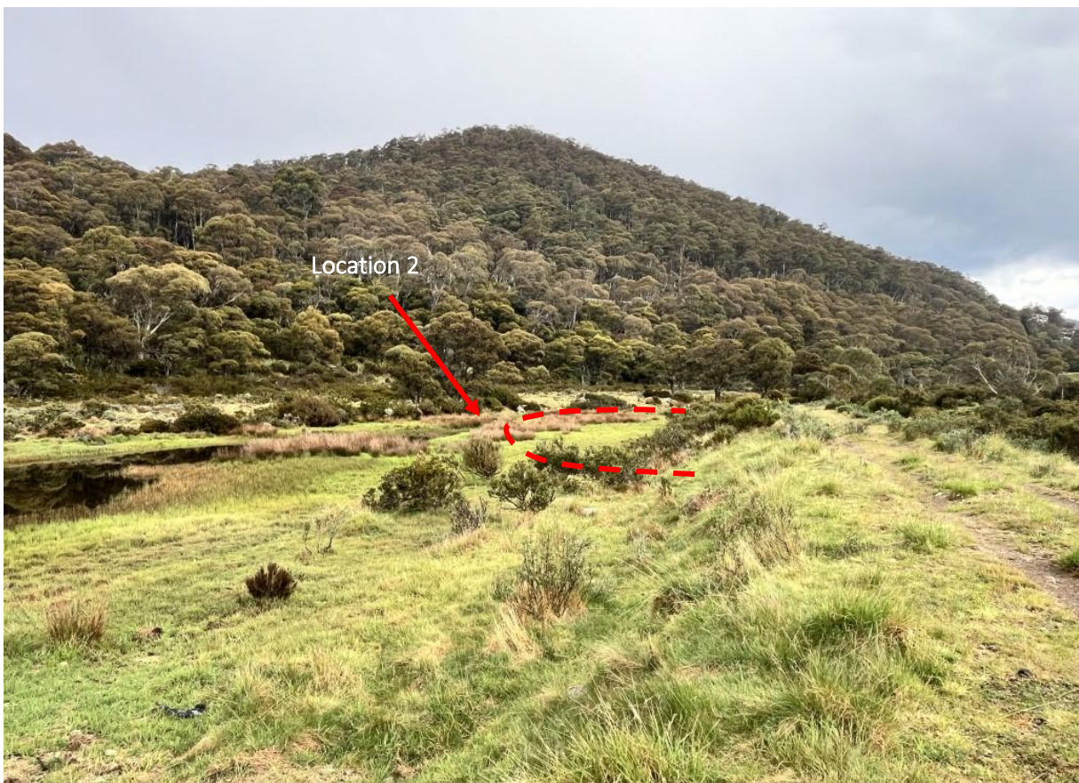
Photo 4: Looking towards Location 2 from the access road. A 15 tonne excavator will descend from the access road and then head south to Location 2. It will then excavate the material from Location 2 placing it on geo-fabric. It will then be loaded by a long-arm excavator located on the access road onto a tipper truck.
